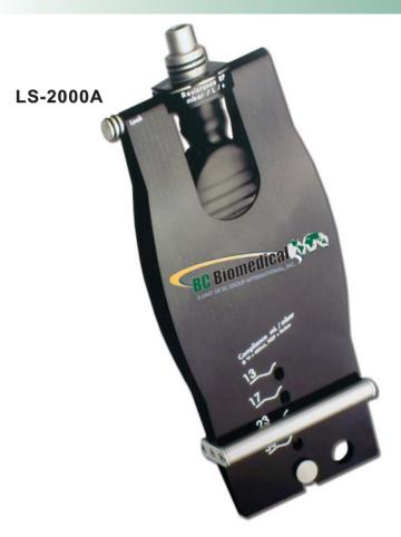
The LS-2000 is an extremely simple concept, as small and portable as a conventional test lung but incorporating an adjustable compliance and a variable resistance feature as well as a leakage control valve to verify the patient-trigger-function or the leak compensation of a respiratory system. Choose between the Adult (LS-2000A) or the Infant Version (LS-2000I).
